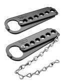
Safety Lockouts provide a means of using multiple padlocks on a secured power source. Manufactured with six station holes. Overall length is 5.06 in. (128 mm) and padlock holes are .38-in. (10-mm) in diameter.
