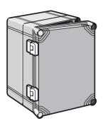
QLine I Hinge Kit includes two polyamide hinges, eight M4 self-tapping plated screws, eight flat washers and drilling template. Use on all QLine I enclosures. Hinge Kit meets Type 4 requirements. Three hinges required for 600-mm sides.
