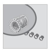
QLine I Brass Inserts are self-tapping brass inserts that fit into molded pads in the bottom of the enclosure. Inserts have an M5 external thread that taps into the molded pad, and an M3 internal thread.
