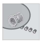
QLine E Brass Insert is a self-tapping Brass Insert that fits into molded pads in the bottom of the enclosure. Inserts have an M2 internal machine screw thread and M4 self-tapping external thread.
