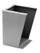
The Floor Stand Kit easily installs on most Wall-Mount or Free-Stand enclosures for floor mounting or elevation. To install, drills holes in the bottom of the enclosure and bolt the floor stands to the enclosure. It is not necessary to remove the wall-mount brackets from the enclosure.
