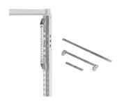
Three sizes of grounding bars and insulated mounting brackets are available. Bars include M6 and M5 tapped holes to provide a common point for grounding equipment. Fits all enclosures if mounted vertically. See table for horizontal mounting.
