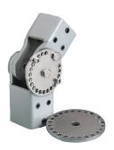
Compact Series 4 Rotation Limiter is an accessory for use with Wall Joint, Cable Wall Joint and Intermediate Joint. It limits the rotation of these joints which normally rotate 180 degrees and provides stops in 15-degree increments.
