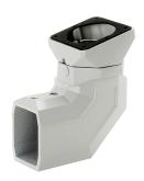
Compact Series 2 Flange Elbow Coupling, 15-Degree attaches directly to the enclosure for applications where a vertical tube is not required, enabling 300-degree enclosure rotation and 15-degree angle tilt. Maintenance-free bearing is steel and polyamide. Includes access plate for easy wire installation.
