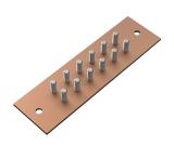
The Ground Buss is a copper bar that features wiring tie points within the cabinet, providing a central grounding point. It mounts on studs provided on the cabinet side. Tie-point spacing is 3/4-in. pair-to-pair and 5/8-in. across each pair. The ground studs are 1/4- $20 \times .75$ -in. on 3/4-in. centers.
