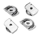
Twenty clamping nuts with top-grip nut retainers. Clamping nuts fit into mounting channels that are used on inside walls of HOFFMAN enclosures. These clamping nuts can be used for mounting other equipment (brackets, etc.) to the enclosure walls.
