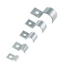
These cable clamps are used when securing cables. They provide the conductivity required to ground the shielding on EMC-shielded cable.
