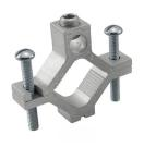
nVent ERICO PermaGround Water and Gas Pipe Ground Clamp is engineered of high-strength 6061-T6 aluminum alloy and are used for connecting copper or aluminum conductors to copper water pipe, galvanized pipe or steel conduit. The conductor and pipe range taking capabilities make this connector ideal for installations requiring long ground wire runs.
