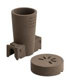
The nVent ERICO Cadweld One Shot 3D Cable to Rebar is a custom, single-use mold using Advanced 3D printing technology to create high-quality permanent exothermic connections. This mold has been designed specifically for cable-to-rebar connections, and its compact size allows connections to be made in narrow or hard-to-reach places. The mold is for single use only and can be quickly installed, making it ideal for making ufer ground connections.
