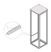
Varistar horizontal cable support rail in the cabinet depth. Mounted directly at the frame.
