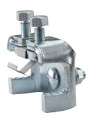
This code-compliant Structural Attachment is part of the nVent CADDY line of innovative rigid bracing system, designed to provide superior performance and meet the highest seismic load requirements. Its innovative design allows quick and easy installation onto both top or bottom flange of a wide range of steel I-Beams. Its snap-off bolts make inspection of seismic sway braces simple.
