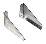
The Equipment Rack Angles can be added to 36-in. and 48-in. tall cabinets for extra 19-in rack equipment mounting. The EIA spaced holes are tapped 10-32. They mount to raised pads on the cabinet back on the inside with the hardware that is provided.
