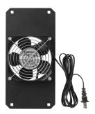
The AccessPlus Fan Kits are a four-inch, 115 VAC solution that provides air flow through cabinets at 100 CFM. The mouning plate and hardware is included. The small mounting plate is  $5.32 (135 \text{ mm}) \times 8.00 (203 \text{ mm})$  and fits cabinets where C = 18.00. The large mounting plate is  $5.32 (135 \text{ mm}) \times 10.75 (273 \text{ mm})$  and fits cabinets where C = 25.00 or 30.00.
