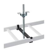
The Cable Runway Center Support Kit is a threaded rod and bracket that supports the center of ladder rack from a ceiling. The kit includes a heavy-duty ladder rack cross member, two mounting brackets, two #12-24 screws, a 5/8-inch threaded rod, a protected sleeve and four 5/8-inch nuts. Supports should be used at least every 5 feet (1.5 m).
