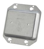
The nVent CADDY Dryer Plug and 2-Gang Protector Plate is an innovative solution designed to safeguard mud ring openings. With an improved installation method featuring a keyhole slot, installers only need to loosen the device screw, position the protector plate and retighten without needing to remove the screw. Designed to fully cover mud ring opening and eliminate drywall mud from entering the box.
