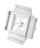
The nVent CADDY Box/Conduit Securement Platform (BCSP) is a fast and secure method to install a wide range of junction and electrical boxes/conduit in overhead installations with a single threaded rod drop. Our improved product is ideal for open ceiling environments with limited access to the structure (high ceilings).
