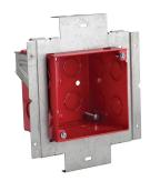
nVent CADDY Fire Alarm Box with Mounting Plate is a powder coated adjustable depth box for mounting fire alarm devices and strobes, designed for on-stud and between stud applications. With two screws inside the box, installers can easily adjust to different depths after installation of drywall or ceiling tiles.
