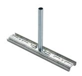
The nVent CADDY WBT Performance Tray Center Support is a simple and efficient way to support wire basket trays from a single threaded rod. The offset center tube helps ensure the tray is centered and secured, enhancing both structural integrity and improving project efficiency. Designed for light-duty cable support projects, installation is easy—simply hold the Center Support parallel to the tray, then turn perpendicular until you hear the Center Support lock into place.
