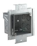
nVent CADDY Adjustable Depth Box with Mounting Plate is a pre-galvanized adjustable depth box for mounting fire alarm devices and strobes, designed for on-stud and between stud applications. With two screws inside the box, installers can easily adjust to different depths after installation of drywall or ceiling tiles.
