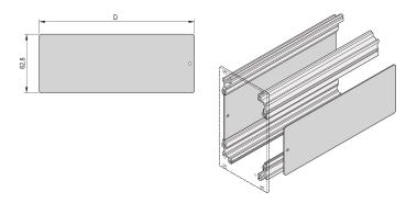
The side Panels can be inserted into the groove of the corner profile.
