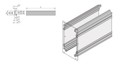
Side Panel corner profile for frame type plug-in unit, PCB depth 160 and 220 mm.
