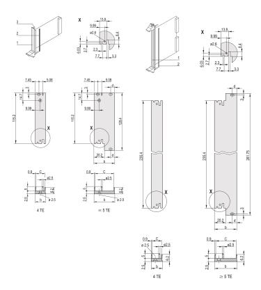
U-Profile front panel can be shielded with a textile gasket. It can be combined with the IEL and IET or the type 2 handle in trapezoid form, PCB mounting = 0,1" offset.
