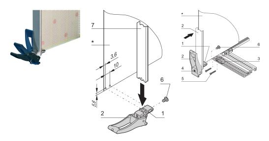
Suitable for insertion and extraction forces up to 1500 N (per pair). Robust board fixing via double bolts. The insertion function will be supported by a keying part which will be assembled onto the horizontal rail.
