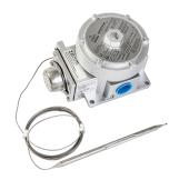
nVent RAYCHEM Raystat-EX-02 is a hazardous area mechanical surface sensing thermostat providing temperature control for heating cables. Switching temperature range -4 °C to 163 °C, adjustable externally to the Ex enclosure by a dial mounted under a bolted-on cover and seal. Switching current capacity is 22 A.
