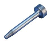
The one-piece D6 mechanical anchor is used when there is not an adequate length of reinforcing bar to be threaded in a standard nVent LENTON threading machine. This anchor is ideal for use in segmental construction when the mating elements have limited space or are severely congested. This system, when combined with the nVent LENTON Form Saver, eliminates hooked bar congestion, protruding dowels and the need to drill holes in expensive formwork.
