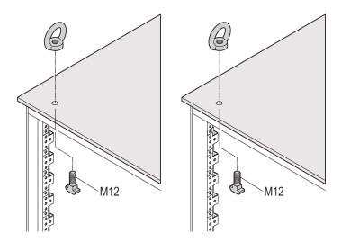
Bolt on lifting eyes to lift and place cabinet without cabinet damage.
