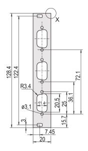
Flat front panel with cutout for D-Sub connectors. Shieldable for stainless steel EMC gasket.
