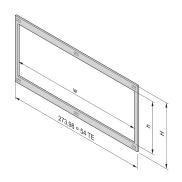
Front frame installation provides the contact between subracks and assemblies. It must be used if a customer has selected a horizontal board mounting Kit.
