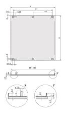
U-profile front panel for textile EMC gasket.
