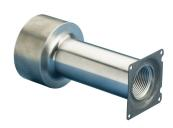
The nVent LENTON Form Saver with Large Anchor provides a method of splicing reinforcing bar in segmental concrete construction applications that have limited space or are severely congested. The large head significantly reduces required embedment length of the mating reinforcing bar.
