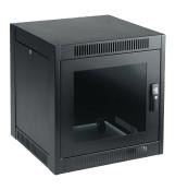
SOHO Cabinets are designed to house servers, networking equipment and phone and voice mail equipment under a desktop. Casters allow the cabinet to be easily moved for access. Equipment is passively cooled by air taken in from the front of the cabinet and expelled through fan cutouts in the rear, which can accept optional fans for warmer applications.
