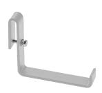
The L-Bracket Kit supports power or other cables that need to be separated from the main cable run. It is made of steel with a painted or plated finish while mounting onto a ladder rack stringer. The kit includes mounting hardware.
