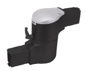
Syspend 180-Max Intermediate Joint joins two horizontal tubes together for a longer length. The arm can be rotated 300 degrees. Includes safety stop and maintenance-free bearings. Use of the intermediate joint reduces the system load rating capacity to 146 lb. (66 kg) at 3.3 ft. (1 m).
