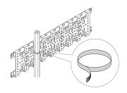
Velcro® Strip is one of the simplest cable bundling solutions. nVent SCHROFF Velcro® strip allows up to 90 mm diameter of wires.
