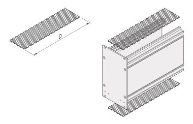
Cover plate for frame-type plug-in units, with perforation guarantee an air flow rate by approx. 65%. The plate is inserted into a groove of the side Panel.
