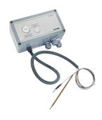
nVent RAYCHEM T-M-20-S is a surface sensing thermostat providing temperature control and temperature limiter in safe areas. Available in 3 temperature ranges. 0-100 °C; 0-200 °C; 50-300 °C.
