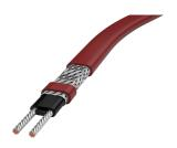
nVent RAYCHEM HTV self-regulating heating cable is designed for freeze protection or process temperature maintenance of pipes and vessels up to 205°C continuously, with a maximum exposure temperature of 260°C. The HTV cable has a solid construction with a high power retention (HPR) heating core and pressure extruded electrical insulation. It is then integrated with a robust metallic braid and a chemically resistant fluoropolymer outer jacket.
