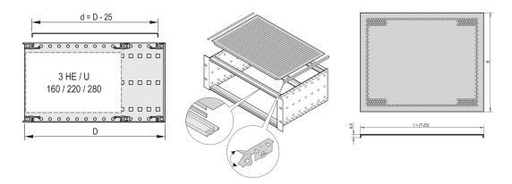
A cover plate is used for electromagnetic shielding or as mechanical protection. The cover can be used is non-standard boards will be assembled into the subrack.
