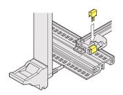
ESD clip can be plugged into the keying/coding block of the guide rail with coding. Provides an conductive contact between the alignment pin of the inserter/extractor handle (IEL or IET) and the horizontal rail.
