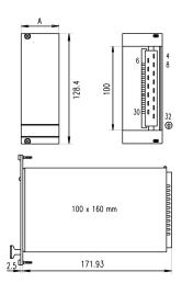
Pluggable 19" Power Supplies with H15 connector for fanless applications. With wide range AC input and three output voltages.
