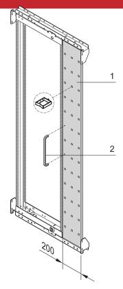
Varistar swing frame provides optimum space usage inside the rack. The swing frames come with handles.
