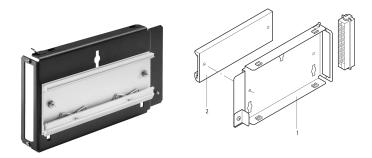
Wall mounting bracket for nVent SCHROFF 19" Power Supplies.
