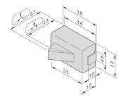
Mirco Switch for AMC Carrier. Option as closer or opener available.
