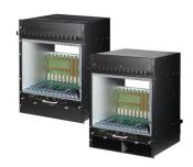
The nVent SCHROFF ATCA 450/40 FC Series is a family of AdvancedTCA Shelves that provide cooling and power per slot for 450 W blades. The backplane is verified in accordance to 40GBASE-KR4 for 40 Gbit Ethernet. Shelves with air flow from bottom to top as well as shelves with air flow from front to rear are available.
