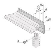
Z-rail for connector in accordance with EN 60603-2 (DIN 41612).
