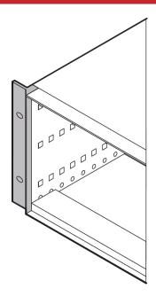
For conversion of Ratiopac cases with cover strip or front handle. The retrofitting of the brackets can be done without disassembly of the case.
